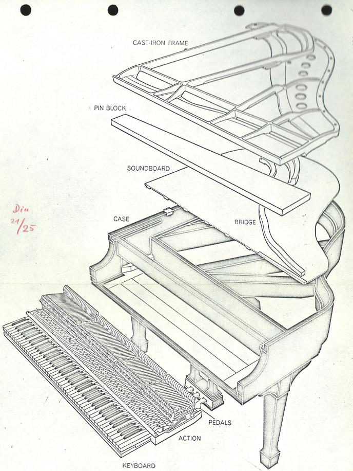
EXPLODED VIEW of the baby-grand piano depicted from above on the preceding page shows the relations of several main components. The keyboard (bottom left) has 88 keys divided into seven and a third octaves. Each octave has eight white keys for playing the diatonic scale (whole notes) and five raised black keys for playing the chromatic scale (whole notes plus sharps and flats). Connected to the keyboard is the action, which includes all the
