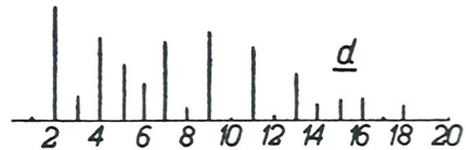
Fig. 5. SEEBECK'S experiment 3 . The pitch of wave form b (400) is an octave above that of wave form a (200). In wave form c a component of pitch 200 is distinctly audible. In wave form d it is even more prominent than the component of pitch 400. The fundamental tone, however, is very weak in wave form c as well as in wave form d .
